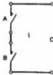
Figure 3b. Contacts in Series. C = A \text{ AND } B
