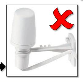
The temperature probe above has NO radiation shield and will likely report erroneously warm temperatures during the day.
