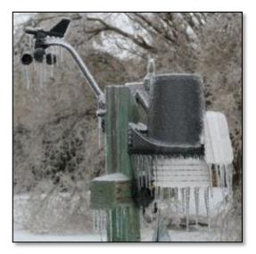
However, both types of anemometers are susceptible to icing. Look for Black-colored anemometers, which will tend to 'thaw out' quicker than white-colored equipment.
