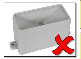
Avoid small rain gauges. The smaller the surface area that collects rainfall – the less accurate the measurement will be.
