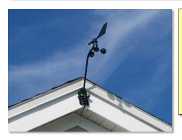
**LEFT:** This anemometer is mounted far too low relative to the roof line. The wind direction will be heavily influenced by the peak of the roof, and the wind speed will be erratic as the roof may enhance or block the wind, depending on the direction.
