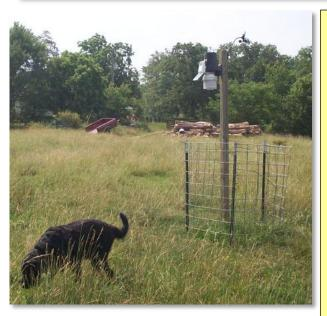
**LEFT:** The temp/humidity sensor is at an ideal height over representative ground cover. The rain gauge is at a good height to avoid dog-watering by the "Weather Lab."
