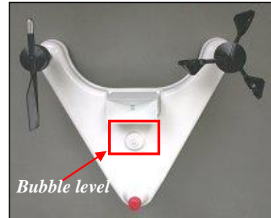
Figure 15: The bubble level (in red box) confirms the station is level, which is required for accurate rainfall and solar radiation measurements.
