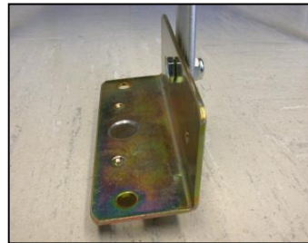
Figure 6: For temporary sites, drive the stakes of the TP1-ST Kit (left) through the center hole in each tripod foot (right). The stakes should be driven in until they barely contact the foot surface. For permanent sites, install user-supplied bolts through the holes in each tripod foot.
