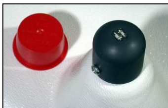
Figure 16: A red or green cap (left) protects the solar radiation sensor (right) while the WeatherHawk is being shipped and installed. Accurate measurements require the cap to be
