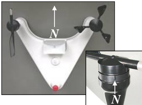
Figure 14: Accurate wind direction measurements require the reference line on the wind direction sensor (right) to be aligned with Magnetic North.
