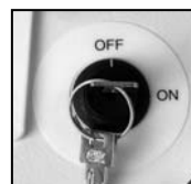
Figure 3: Keyed power switch is located on the bottom of the WeatherHawk station.
