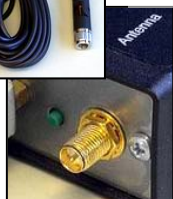
Figure 10: The connector labeled Antenna on an RF400-series radio is where the antennas attach.
